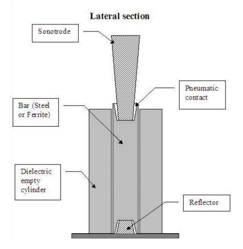
Fig 1: Experimental set-up. Lateral section.
