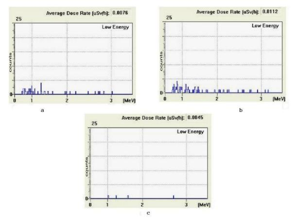
Fig 2: (a) Neutron spectrum from the bar of Ferrite - (b) Neutron spectrum from the bar of steel - (c) Neutron spectrum of the background. For all of them we have MeV on the abscissa and counts on the ordinate
