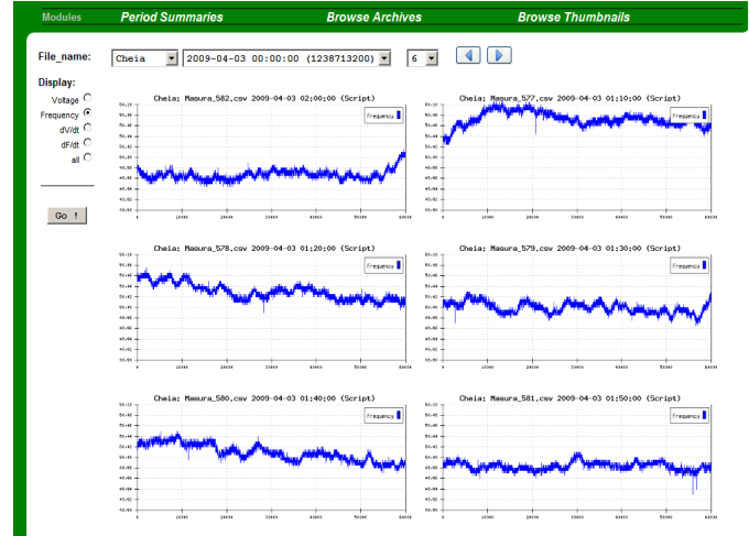
Fig. 5. Frequency variation for 60 minutes MOT registration in April 2009
